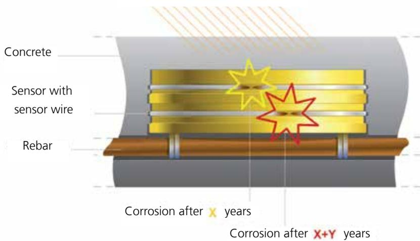
wireless-readable sensor-transponder; with that it is possible to fit the sensor into the construction without »harming« the surface. The energy required for the measuring is harvested from an electromagnetic field, thus batteries and their exchange are unnecessary – the transponder can remain permanently inside the construction, while the measured data is transmitted via radio to a reading device.
